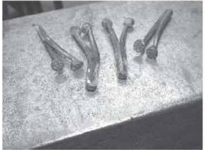
Each pair of flowers started as 2 inches of 1/4 round. Neck down just inside the very ends, draw out the stem between the ends less than 3/16, then texture the ends with a punch.
