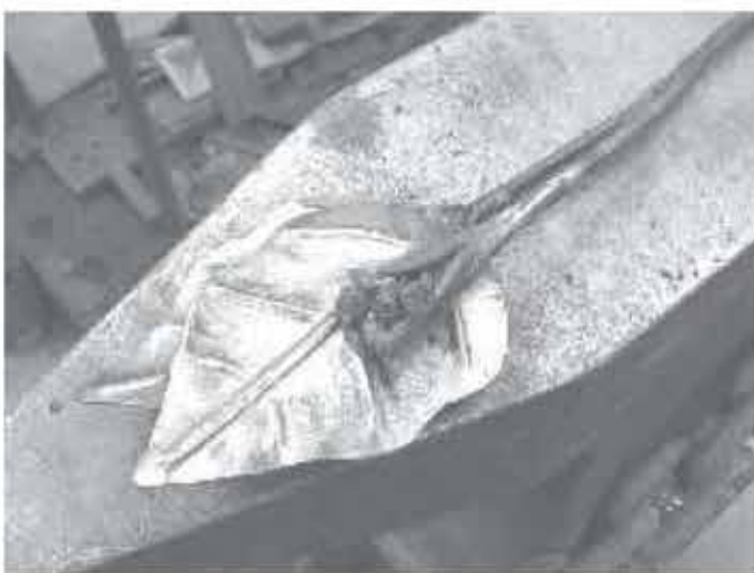
Weld leaf stems to the main stem. leaving room for bracts.
