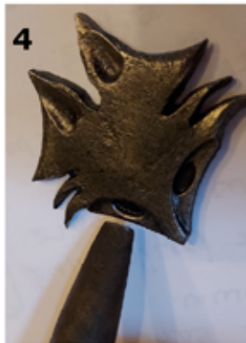
1. Finished Fox! 2. Marking material. 3. Layout of face. 4. Eye punch is shaped like a football. Note: Cheeks are ground slightly to give personality to fox. 5. Layout cuts on bar. Easier to work with bar attached, then cut off when necessary. 6. Tool made for creating cheek depressions.
