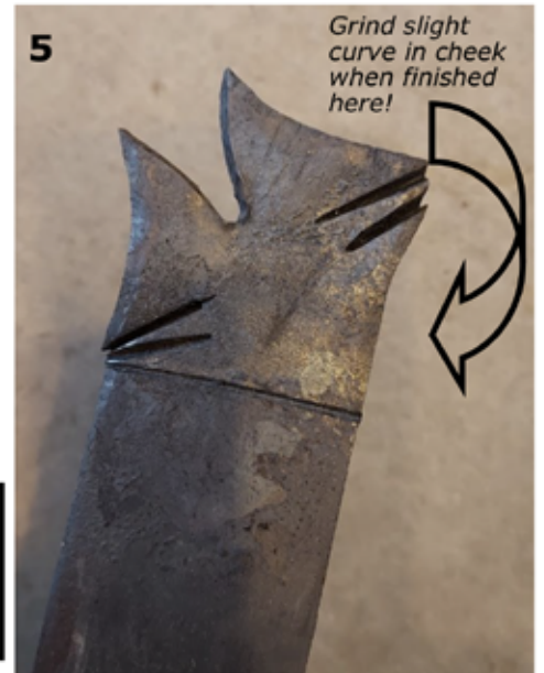
1. Finished Fox! 2. Marking material. 3. Layout of face. 4. Eye punch is shaped like a football. Note: Cheeks are ground slightly to give personality to fox. 5. Layout cuts on bar. Easier to work with bar attached, then cut off when necessary. 6. Tool made for creating cheek depressions.
