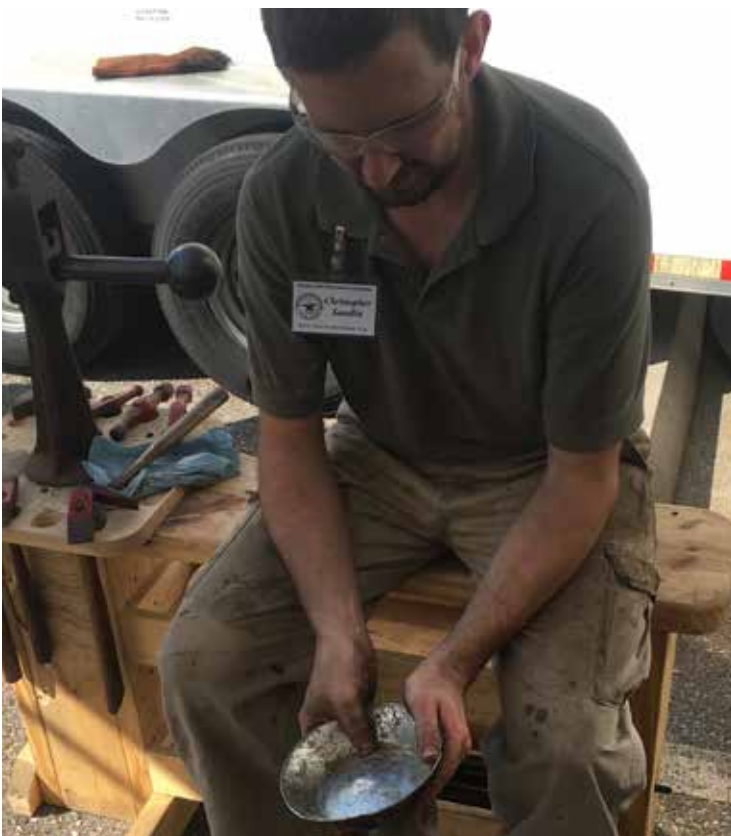
Christopher Sandlin sitting on his coppersmithing workbench while tinning a copper pan. Next year at FABA CON 22, Christopher plans to demonstrate several aspects of coppersmithing.
