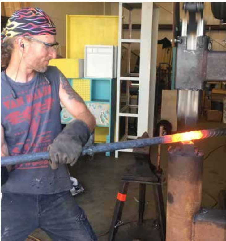
Jeff Badarak using the FABA power hammer to dress up some rebar that he's using in a staircase project.
