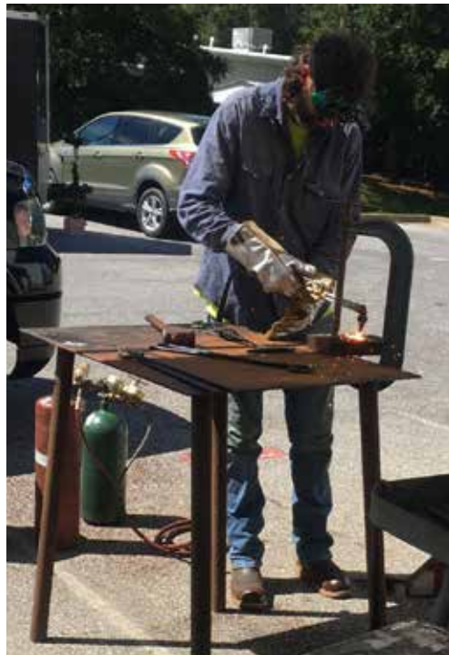
We needed a punch plate to drift the hammer through so Brien Byerley used a torch to make one. Dirty but functional. (NOW that's a clamp!)
