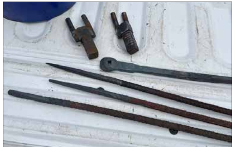
Alvin's new nail header (spike size), two hardy bending forks and rebar practice pieces.
