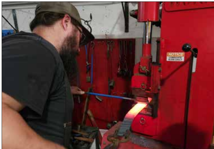
William pressing on with drawing out a large bearing race.
