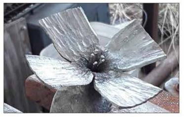
round chisel. If I'm making a dogwood blossom, I also melt a small notch in the center of the end of each petal. This is not necessary or desirable for most flowers.
