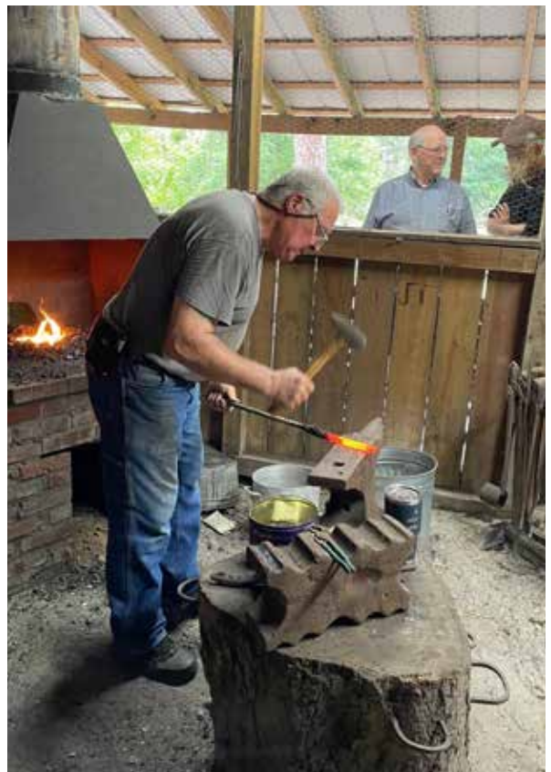
Trez Cole demonstrates making damascus and a knife blade.
