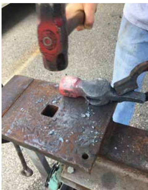
James (above) watches the heat for his boarding axe. The boarding axe was made from a 2.5-pound Harbor Freight ballpeen hammer (left). The FAB power hammer became very useful for this project.
