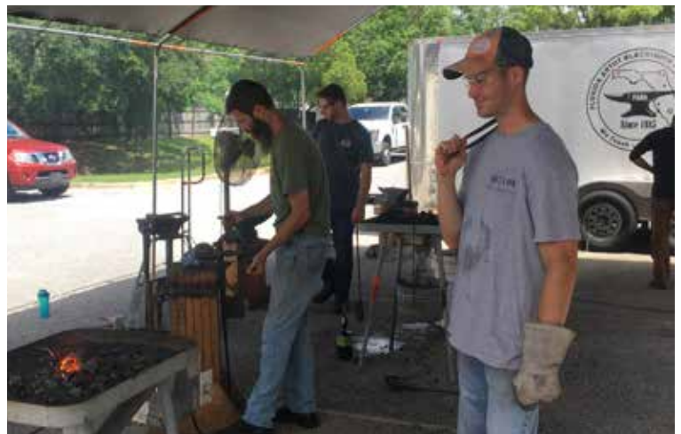
James (above) watches the heat for his boarding axe. The boarding axe was made from a 2.5-pound Harbor Freight ballpeen hammer (left). The FAB power hammer became very useful for this project.
