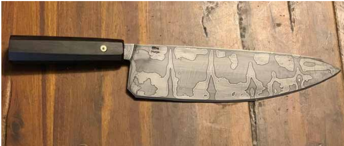
Marcus Wise has again been making some spectacular knives. He made this 10" Damascus chef knife from 1095/15n20 with an integral bolster and African Blackwood handle.
