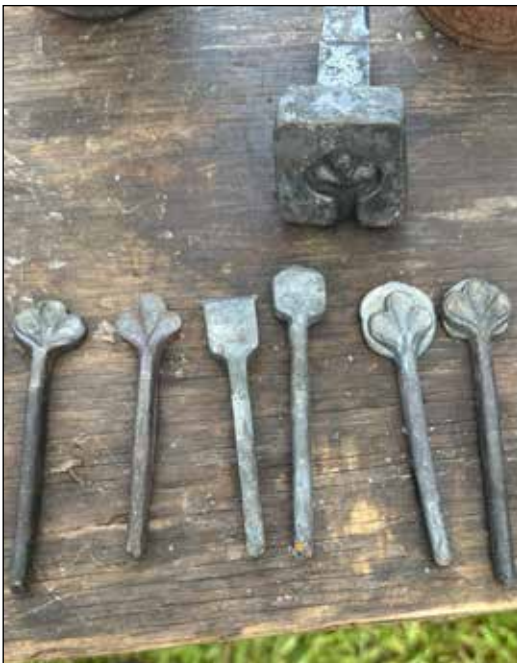
Some of the tools and dies that Bradley Schwartz made at SBA. They are used to make positive and negative repeating elements in metalwork.
