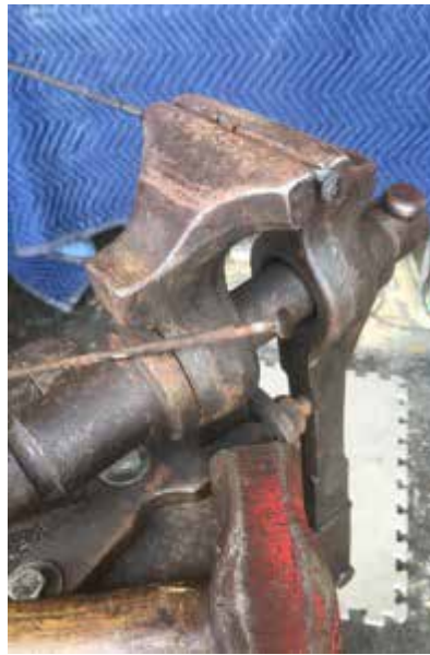
We used the post vice as a bolt header. The original (lower bolt head) was a 16-inch-long carriage bolt.
