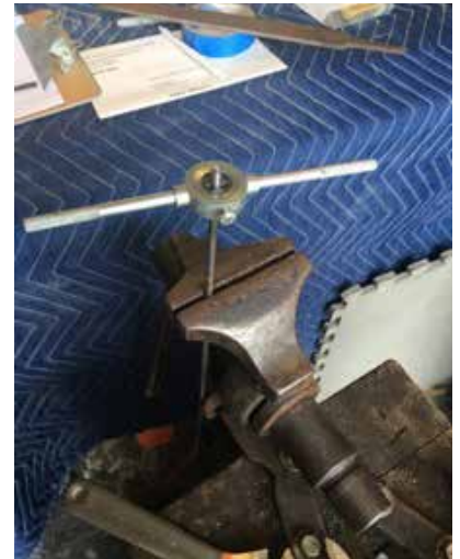
Cutting threads (yes, that is a copy of Clinker Breaker on the workbench in the background)
