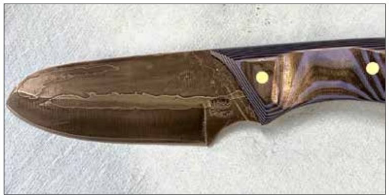
Marcus Wise - has again been making some spectacular knives. He finished up this San mai hunter with G10 scales and brass pins for a knife collector that just wanted something "different". Also tune into the history channel on Wednesday February 17, 2021 at 9pm eastern time to see Marcus compete against 3 other bladesmiths in Forged in Fire!
