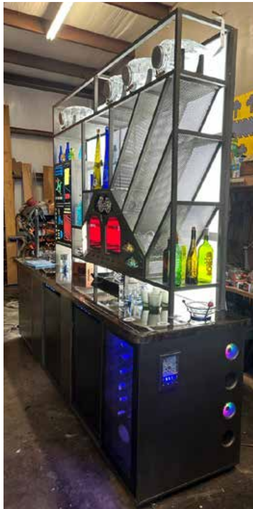
Bottom filling beer dispenser, automatically turns off when it reaches full.
