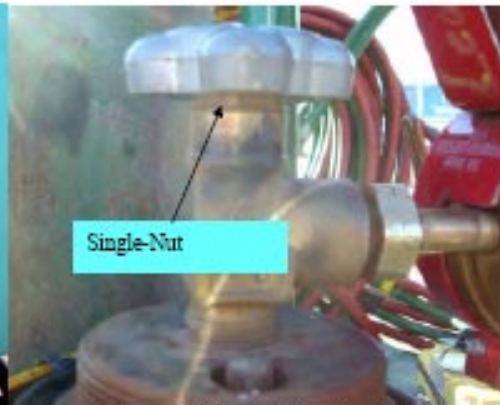
Figure 2. A non-leaking shutoff valve with a single-nut configuration
