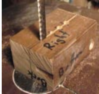
Figure 2: Initial hinge cut
