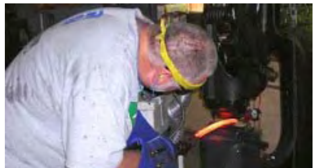
Gary forging out the billet to 2x the length
