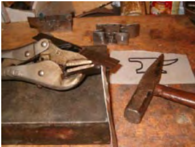
Utilizing the vise grips and the hammer begin bending the sheet metal to the desired shape.
