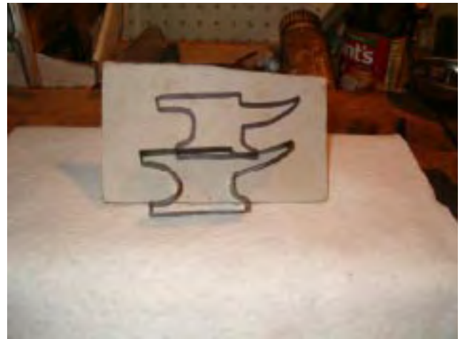
Compare your cutter with the drawing and if not satisfied refine the shape.
