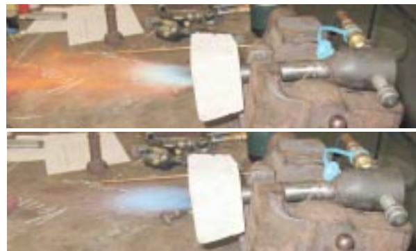
Figure 11: Tuning a bell burner
