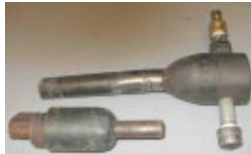
Figure 1: A "Bell" burner
