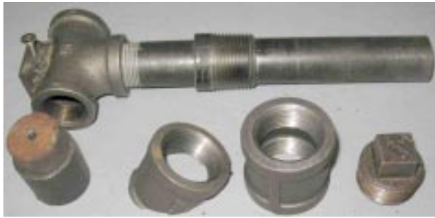
Figure 12: Burner mounting hardware
