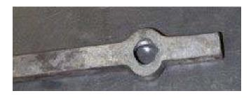
Start by figuring out how wide a chisel you should use. Francis Whitaker worked out a formula for calculating this. Use 89% of half of the circumference of the round hole.  $\frac{1}{2}$  hole = .89 x ((2 x 3.14 x  $\frac{1}{4}$ ") / 2) = 0.7" wide chisel The chisel should have sharp sides slightly tapering in so that the chisel will cut a clean slot and not punch out a slug.
