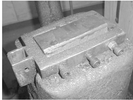
Figure 1: Removable hardy hole
