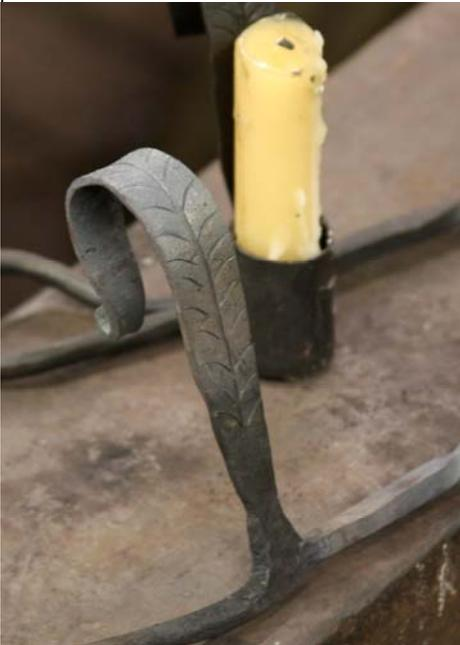
8. Decorate the handle as desired, scroll a small loop on the tip, and then form a Sheppard's crook of about 1" diameter.
