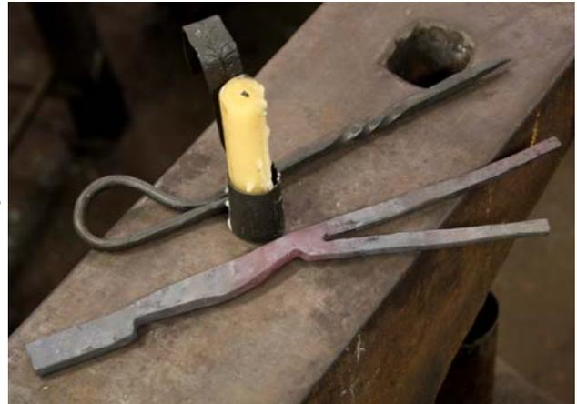
3. Shoulder the top edge of the piece 2" from the end, and 1/2" from the end of the slit. Use the far edge of the anvil for the first shoulder and the near edge of the anvil for the second. These two shoulders will define the start and end of the section that will become the loop handle for the lamp.
