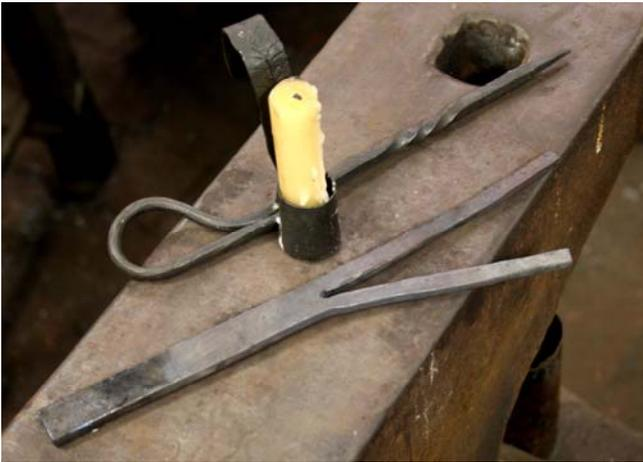
2. Clean up the rough edges of the slit if needed with a file, and roughly square and straighten one side of the slit. This creates a clean piece of steel to hold with the tongs for all the work to follow on the other end of the stock. This squared off fork will become the pointed stick part of the lamp. This straight fork of the split I will call the bottom edge of the lamp.
