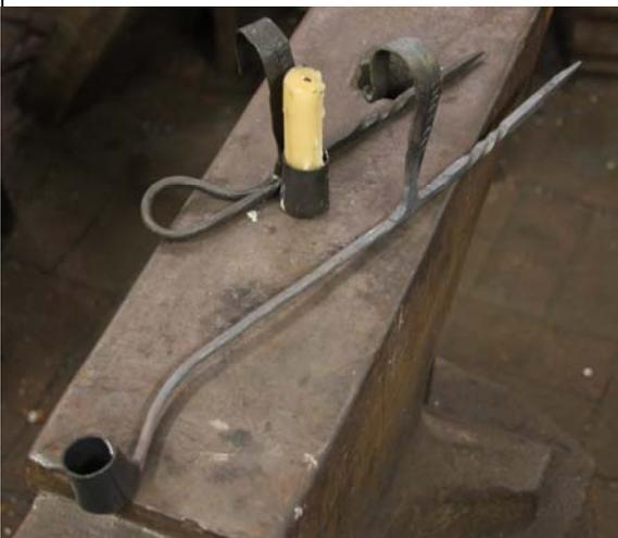
10. Roll the cup to make a round tube – adjust to fit whatever candle you intend to use. Note the direction of the roll! It should roll the same direction that you rolled the handle (I call that toward the back of the lamp).
