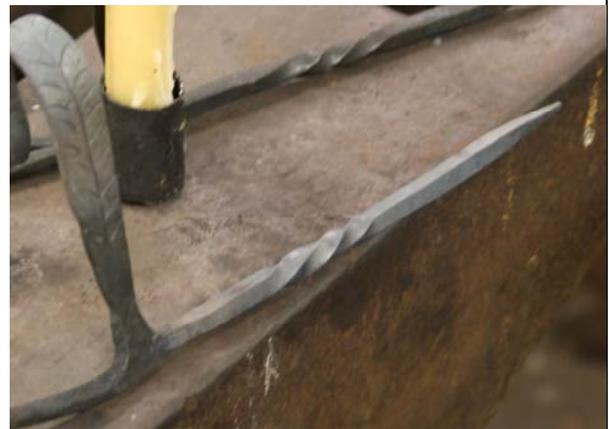
9. Draw out the other fork from the split to a 1/4" square about 6" long, taper the tip, and add a decorative twist. I used a 3/4 turn twist. Note that the spike is left square, whereas the loop handle was rounded.
